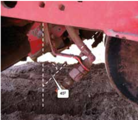
Correct positioning of the nozzle 45-55 degrees from the vertical
