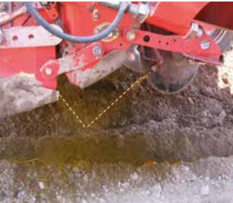
The intersection of the axes of the spray - is the optimal location
